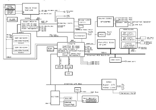
Figure 1-3 System unit block diagram
